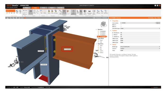
We have imported, designed and code-checked a steel joint according to AISC.
