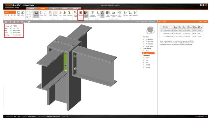
Activate **Overall check, Equivalent stress, Mesh** and **Deformed** from the ribbon to get a full picture of what is happening in the joint. Everything is displayed in the 3D window.
