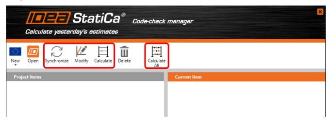
Code-check manager is a BIM tool to export and synchronize connections from other programs. It is launched directly in the 3rd party applications via a command/icon.
