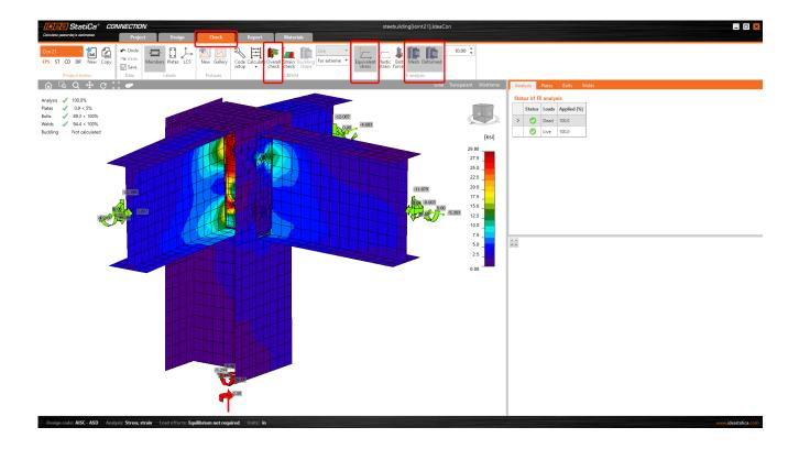
All values can be reviewed in detailed in the tables and 2D window. For example, to display check of bolts select tab **Bolts** tab.
