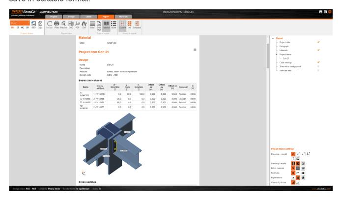
We have imported, designed and code-checked a steel joint according to AISC.
